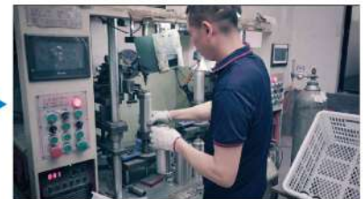
6. Seamless welding the top and base
