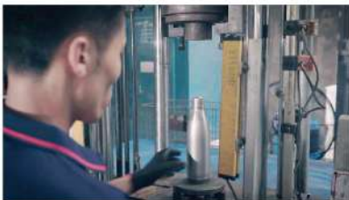
4. Molding shape the bottom and top
